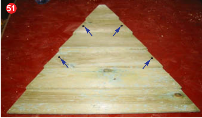
51 Drill 4 holes in the 6 small triangular roof panels.
