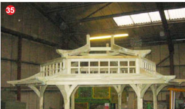
Lift bearer assembly onto uprights and align with the uprights.
