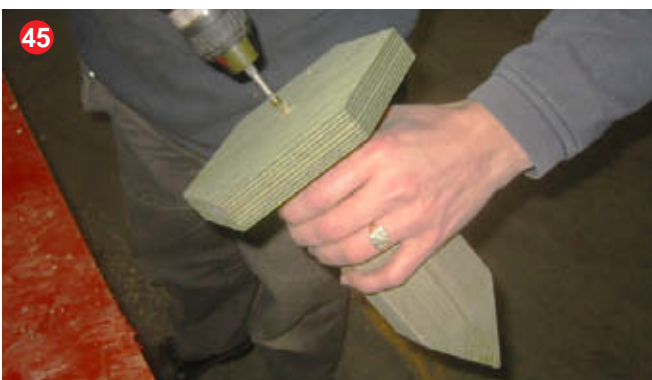
Centrally attach the 2nd hexagonal piece to the centre finial using 1 x 70mm screw.
