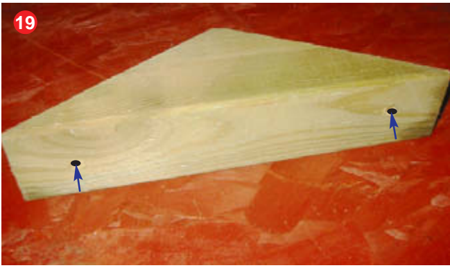
19 Drill 2 holes in each of the triangular corner supports.
