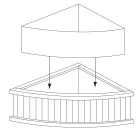
**Top planter:** Use 6 x 15mm tacks to hold the edge of the liner in place
