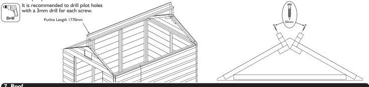
Secure to each felt batten one large roof panel and one small roof panel using 10 x 30mm nails as shown. Ensure the felt batten is flush to the edges of the panels. Position the roof panels onto the assembly, make sure the top edges are located at the apex and the roof is flush with the front and back apex. Secure with 12 x 38mm screws per roof section, screw through the roof and into the panel framing and purlins.
